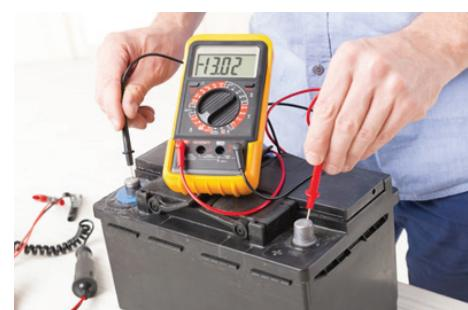
Fig. 2.2.3: Measuring the battery's terminal voltage using a multimeter
