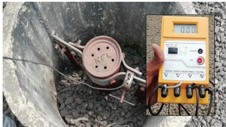
Fig. 2.1.12: Earth resistance measurement
