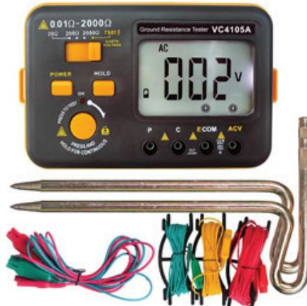
Fig. 2.1.11: Ground resistance tester
