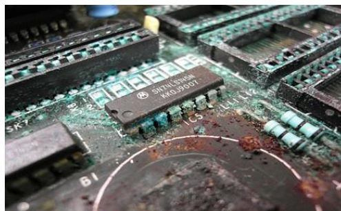
Fig 1.4.6: Metallic filaments on a PCB
