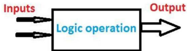
Fig 1.3.42: Symbol of a logic gate
