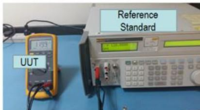
Fig 2.1.7: Sample of calibration test
