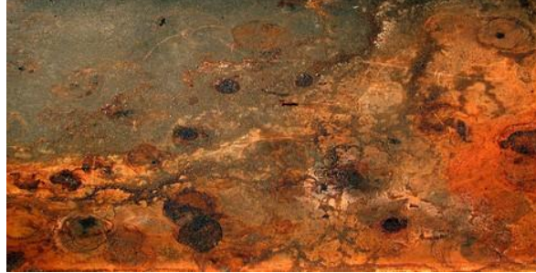
Fig 1.4.7: Moisture coating on a PCB
