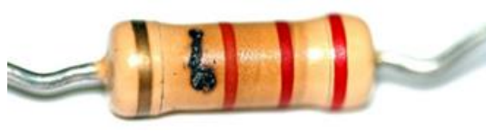
Fig 1.4.8: ESD discharge on a resistor
