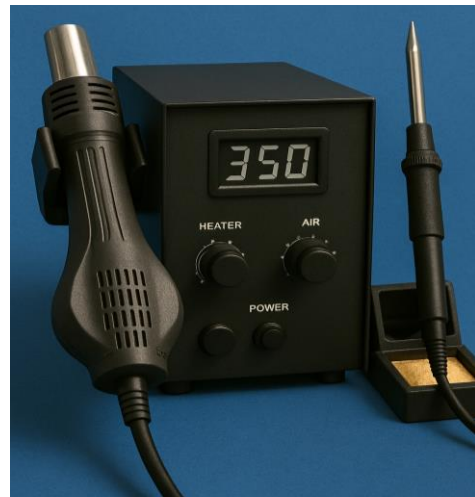
Fig. 2.2.1 SMT Rework Station
