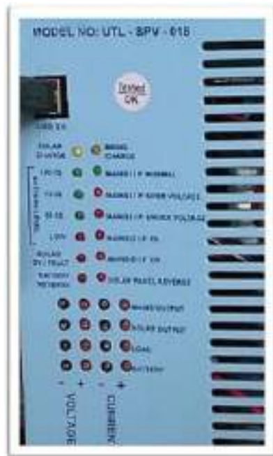
Fig. 7.3.2. CCU Monitoring Panel
