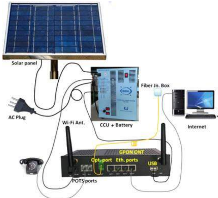
Fig. 3.7.0 ONT Connectivity at Gram Panchayat (GP) level
