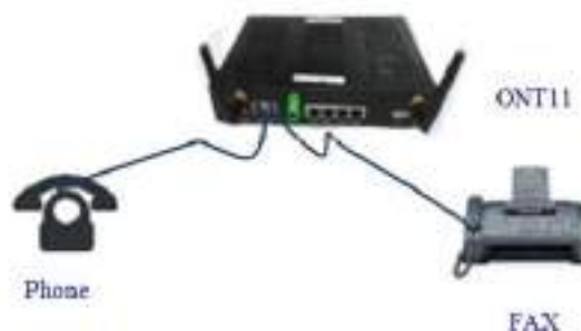
Fig. 3.13.9. Phone / FAX connection for Voice & FAX Service
