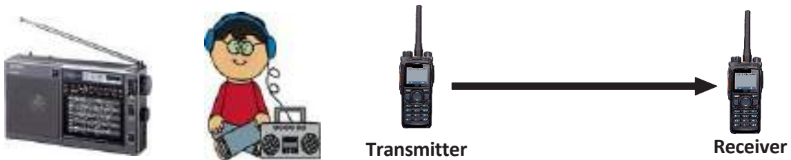
Fig. 1.1.3. Simplex system –Radio Transmission
