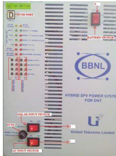
Fig. 7.3.3. Hybrid SPV Power System for ONT
