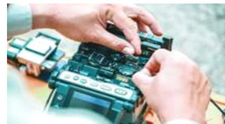
Fig. 1.1.6: Splicing of Optical Fibre
