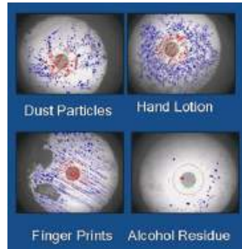
Fig. 3.2.1: Contamination on fibre optics
