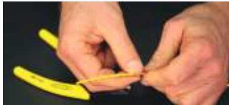
Fig. 3.1.2: Preparing fibre for mechanical splicing
