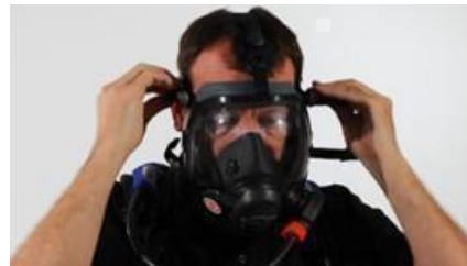
Wear the mask slowly by resting your chin in the resting cusp and pull the head strap slowly over your head.
