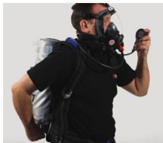
Slowly close the cylinder valve without leaving the knob.
