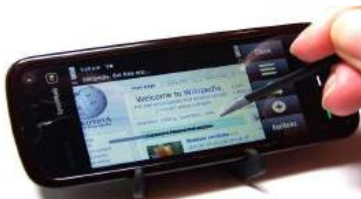
Fig. 1.6.2(iv) Shows Nokia 5800 Xpress Music which was launched in November 2008. The phone had GSM/HSPA network technology and had a Symbian V9.4, Series 60 Operating system. The phone had a TFT touchscreen and was equipped with handwriting recognition.
