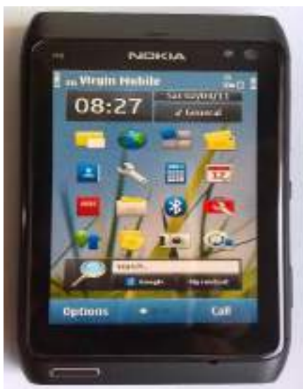
Fig. 1.6.2(i) Shows Nokia N8 which was launched in October 2010. The phone had GSM/HSPA network technology and the operating system installed in it was Symbian 3rd Edition. The phone supported a 16 MP rear camera
