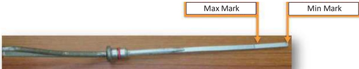
Fig. 2.5.7(vi) Lubrication System Maintenance
