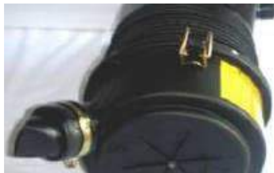
Fig. 2.5.7(iii) EVACUATOR VALVE
