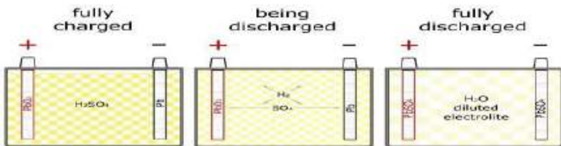
Fig. 2.2.11(i) Stages of a battery
