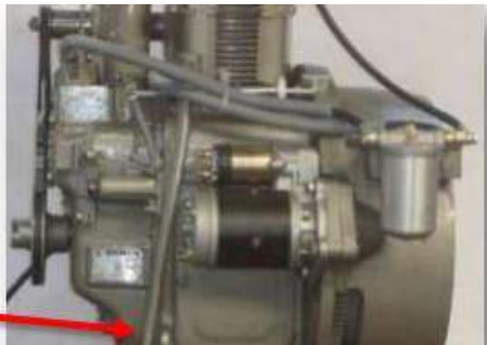
Fig. 2.9.11(iii) Inspection Cover of a DG
