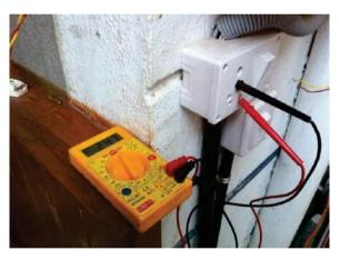
Fig 2.6.5: Connect black test probe to earth outlet
