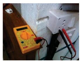
Fig 2.6.3: Connect multimeter knob
