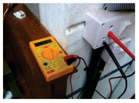
Fig 2.6.6: Red probe and black in earth and neutral respectively
