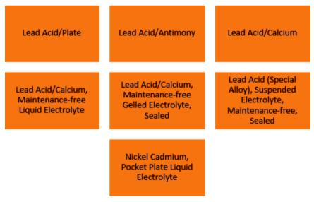
Fig. 2.10.1: Batteries, used for UPS
