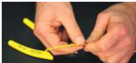
Fig. 3.1.2: Preparing fibre for mechanical splicing
