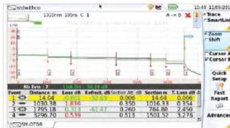
Fig. 4.1.4: OTDR Trace view
