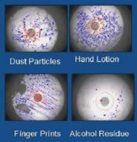
Fig. 3.2.4 (a): Contamination on fibre optics
