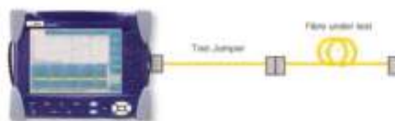
Fig. 4.1.8: Optical return loss test
